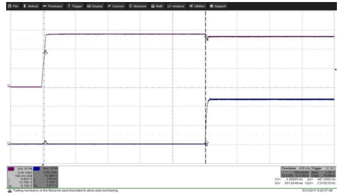
Figure 29: Turn-on by V_{in} transient (ON/OFF high) at full rated load current (resistive) at V_{in} = 44V . Top trace (C2): Input voltage V_{in} (5 V/div.). Bottom trace (C4): Output voltage (5 V/div.). Time: 100 ms/div.
