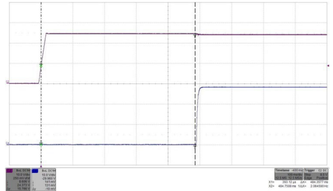
Figure 41: Turn-on by V_{in} (ON/OFF high) transient at full rated load current (resistive) at V_{in} = 24V . Top trace (C2): Input voltage V_{in} (10 V/div.). Bottom trace (C4): Output voltage (10 V/div.). Time: 100 ms/div.
