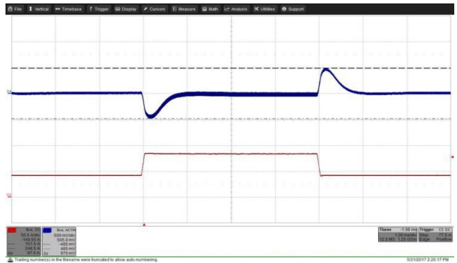
Figure 31: Output voltage response to load current step change 50% - 100%- 50% (42A–84A–42A) with di/dt = 1A/\mu s at V_{in} = 14V . Top trace (C4): Output voltage (500 mV/div.). Bottom trace (C3): Load current (50A/div.). Time: 1ms/div.
