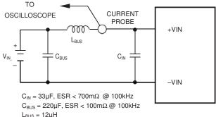
Figure 2. Measuring Input Ripple Current
