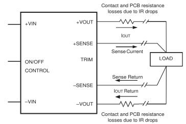
Figure 4. Remote Sense Circuit Configuration
