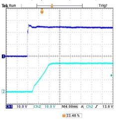
Power On Startup Delay (Vin=0 to 24V, Vout=nom., lout=2A,  $C_{load}$ =0  $\mu$ F, Ta=+25°C., ScopeBW=20MHz) Trace 1=Vin, Trace 2=Vout
