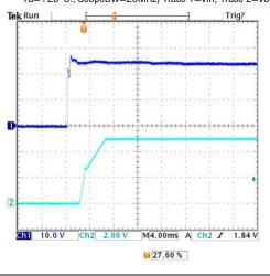
Power On Startup Delay (Vin=0 to 24V, Vout=nom., lout=10A,  $C_{load}$ =0  $\mu$ F, Ta=+25°C., ScopeBW=20MHz) Trace 1=Vin, Trace 2=Vout
