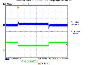
Power On Startup Delay (Vin=0 to 24V, Vout=nom., lout=no load,  $C_{load}$ =0  $\mu$ F, Ta=+25°C., ScopeBW=20MHz) Trace 1=Vin, Trace 2=Vout
