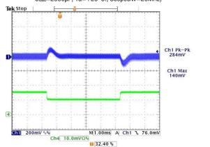
Power On Startup Delay (Vin=0 to 24V, Vout=nom., lout=no load,  $C_{load}$ =0  $\mu$ F, Ta=+25°C., ScopeBW=20MHz) Trace 1=Vin, Trace 2=Vout
