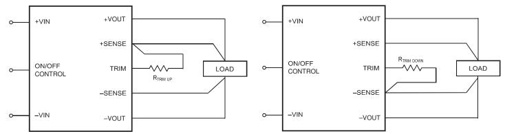
Figure 6. Trim Connections To Increase Output Voltages
